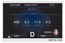
Start engine, pictures and text prompts will be displayed on information display area and blue coolant temperature indicator will come on, it indicates that engine is in warming up status currently; After engine coolant temperature is increased, pictures and text prompts will be displayed on information display area and blue indicator will go off, it indicates that warming up of engine is completed currently.
