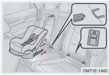
Step 3: Insert and secure lower hook of child restraint system to lower retaining ring.
