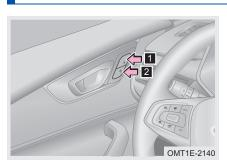
In the vehicle, press unlock/lock switch to unlock/lock doors.
