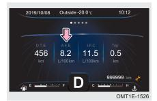
Display average fuel consumption after engine starts. Before that, the meter displays current value.
