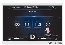
Driving mileage: The estimated maximum distance that can be driven with current remaining fuel (common unit: km).
