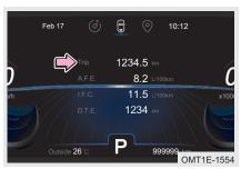
Trip mileage: It is convenient to calculate the mileage for each trip after resetting (common unit: km); The display range is 0 to 9999.9 km. It will return to zero and restart calculation if it exceeds 9999.9 km.
