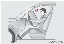
In a event of a severe frontal collision, driver airbag and front passenger airbag work together with the seat belt to help reduce injuries to the head or chest of driver and front passenger caused by hitting the interior component. The front passenger airbag may be activated even there is no passenger in the front seat.
