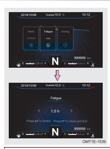
Fatigue driving can be set by operating steering wheel combination buttons:
