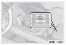
Step 1: Lay smart key in auxiliary fascia console armrest box (as shown in figure) with front side facing up. At this time, do not depress brake pedal (vehicle with automatic transmission) or clutch pedal (vehicle with manual transmission);
