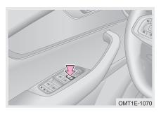
Operate using switch: When vehicle power is turned to ON mode, press outside rear view mirror folding switch to fold mirrors automatically, press the switch again to extend mirrors automatically (do not fold manually).
