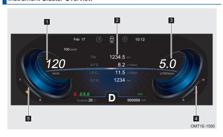
1 Speedometer 3 Tachometer 5 Fuel gauge
