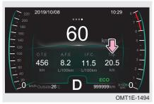
Trip mileage: It is convenient to calculate the mileage for each trip after resetting (common unit: km); The display range is 0 to 9999.9 km. It will return to zero and restart calculation if it exceeds 9999.9 km.
