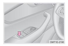
Press passenger side window OFF switch, passenger side window OFF switch indicator comes on and the power child lock is locked, as well as disable passenger side window switch. Press the switch again to cancel this function and the indicator goes off.
