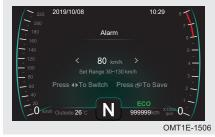
The speed limit can be set by operating steering wheel combination buttons:
