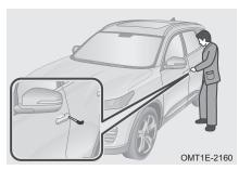
Step 1: Insert mechanical key into hole under left front door handle cover. Turn the key upwards to pry the cover.
