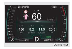
When speed reaches the set value, alarm icon "a" will be displayed on driving information display screen (specific set speed value will be displayed in the icon) and alarm buzzer sounds. Alarm icon and sounds will disappear only when speed is lower than setting value by 5 km/h. If speed reaches the set value again, it will alarm again.
