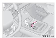
■ Applying parking brake manually With vehicle power switches to ON mode, or engine starts and vehicle stationary, when pulling up the electric parking brake button, red indicator "(p)" on instrument cluster and electric parking brake button indicator will come on, indicating parking brake function has been turned on.
