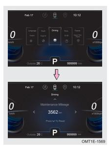
Maintenance mileage can be reset by operating steering wheel combination buttons:
