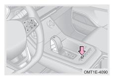
Press lane assist system switch to switch LDW/LKA/OFF circularly.
