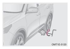
Step 4: When the notch of jack contacts correct jacking-up point, fit jack rocker into jack, and wheel bolt wrench into jack rocker, and turn the wheel bolt wrench clockwise to jack up the vehicle;
