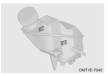
Brake fluid level should be between the "MIN" and "MAX" marks. If the level is in the "MIN" mark or below, add brake fluid and contact Chery authorized service station for inspection and repair immediately.
