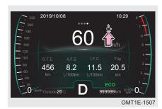
When driving time exceeds the set time, "Driving time exceeds--h, take a rest" will be displayed on information display area, at the same time, alarm sounds for 1 second and fatigue driving icon displays " to inform the driver to take a rest.
