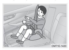
For the expandability of child restraint system function, a separate booster cushion can be used. When the child is shorter and lighter, a booster cushion can be used to increase the child's line of sight in vehicle and secure child properly. (Vehicle seat belt that meets international standards is designed according to body size of person over 1.5 m. If any one under 1.5 m uses seat belt, the belt could hurt his/her neck seriously in case of
