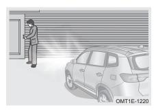
Turn vehicle power to OFF mode, pull the headlight combination switch towards steering wheel side and release, the follow me home function is activated. The low beam lights and position lights will come on. Each time the headlight combination switch is operated, the low beam lights and position lights will turn on for 30 seconds, which can be activated up to 8 times continuously.
