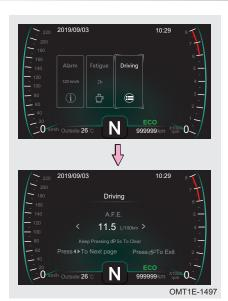
Average fuel consumption: amount of fuel used for mileage (common unit: L/100 km).
