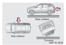
Driver airbag and front passenger airbag may not deploy generally if the vehicle is subjected to a side or rear collision, turnover or low speed frontal collision.
