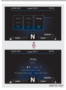
Average fuel consumption: The amount of fuel used for mileage (common unit: L/100 km).
