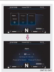
The speed limit can be set by operating steering wheel combination buttons:
