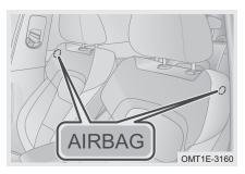
When vehicle is subjected to side collision and deployment conditions are met, front seat side airbag of impacted side deploys. Besides seat belt, front seat side airbag is a kind of device that can provide more protection for driver and front passenger.
