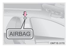
When vehicle is subjected to side collision and deployment conditions are met, curtain shield airbag can provide head protection for passengers sitting on front seat and rear outside seat of impacted side, reducing risk of injury.
