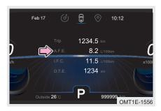
Display average fuel consumption after engine starts. Before that, the meter displays current value.
