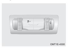
Press ESP OFF switch (if equipped) to turn off ESP; Press the switch again to turn on ESP.
