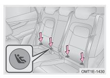
Step 1: Find the lower retaining ring used to secure child restraint system;
