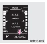
Total mileage: Total mileage of the vehicle (common unit: km); The display range is 0 to 999999 km. It remains 999999 km if beyond the range.
