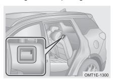
Adjust height of seat head restraints, remove them if necessary and fold up center armrest. Then pull the left seatback adjustment handle forward and pull seatback forward to fold it down slowly. This can enlarge the luggage storage space.
