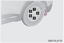
Step 4: Using wheel bolt wrench, tighten bolts in sequence shown in illustration. Repeat the process 2 to 3 times to ensure that wheel bolts are tightened in place;
