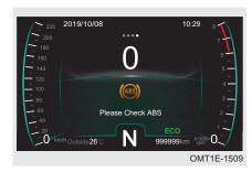
When on-board computer detects that the system is malfunctioning or its information is abnormal, the alarm information will be immediately displayed in information display area one by one and recorded in fault information screen after switching vehicle power to ON mode.
