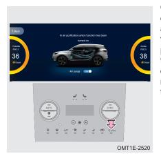
Operate the anion button on the air conditioning control panel to turn on anion and one-button purification functions at the same time. Compared with the single one-button purification function, the air purification efficiency is higher and the air environment quality in the car is better after the anion function is added.
