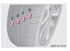
Check the tire tread for tread wear mark. When tread wear reaches its limit, tread will be in the same plane as the wear band. If such condition occurs, it indicates that performance and safety of tire seriously decrease, and replacement is necessary.
