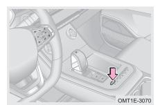
If NORMAL mode is not equipped, system is ECO mode by default when engine starts. Press drive mode switch, switch between SPORT mode and ECO mode circularly. You can choose according to different road conditions.
