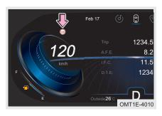
After speed limit sign is recognized by SLA, "100" indicator in instrument cluster comes on, if the speed exceeds current speed limit for 5 km/h, prompt sound will sound 1 time.
