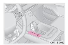
During the operation, the driver can choose the automatic mode (P, R, N, D) and the manual mode M (+, -). The selected gear position will display the corresponding gear information on the information display area in instrument cluster.
