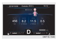
When speed reaches the set value, alarm icon "@" will be displayed on driving information display screen (specific set speed value will be displayed in the icon) and alarm buzzer sounds. Alarm icon and sounds will disappear only when speed is lower than setting value by 5 km/h. If speed reaches the set value again, it will alarm again.
