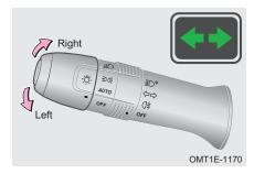
Turn vehicle power to ON mode, switch headlight combination switch: Pull up: Right turn signal light comes on.
