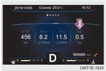
Trip mileage: It is convenient to calculate the mileage for each trip after resetting (common unit: km); The display range is 0 to 9999.9 km. It will return to zero and restart calculation if exceeds 9999.9 km.
