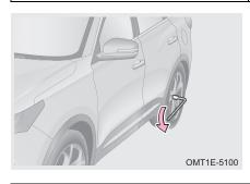
Step 2: Fit wheel bolt wrench to the wheel bolt of flat tire, set the handle on left side, hold the end of wrench handle and push it downward, loosen each bolt of flat tire about one-half turn;
