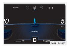
Start engine, pictures and text prompts will be displayed on information display area and blue coolant temperature indicator will come on, it indicates that engine is in warming up status currently; After engine coolant temperature is increased, pictures and text prompts will be displayed on information display area and blue indicator will go off, it indicates that warming up of engine is completed currently.
