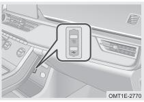
For some models, USB port is located in auxiliary fascia console storage box.
