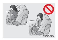
Always keep airbag inflation path clear. It is forbidden to place anything (mobile phone, etc.) between the occupant and the airbag. It is forbidden to fix or place any object on or near the airbag cover. If there is an object between occupant and airbag, the airbag may not deploy according to design path, or the airbag may push object to occupant's, which could result in death or serious injury.
