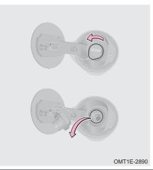
Step 2: Turn fuel filler cap counterclockwise to remove it;
