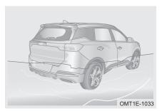
The vehicle could be seriously damaged when driving on a road that has flooded after heavy rain. If driving through water is unavoidable, check the depth of the water and drive slowly and carefully.
