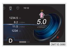
If the vehicle battery is powered off and reconnecting or starting, due to the initialization of electric steering system angle, the yellow indicator "A!" on instrument cluster flashes, turn the steering wheel left and right to the limit position to complete the angle reset, and the yellow indicator " on instrument cluster turns off.
