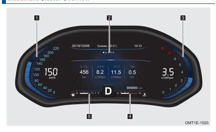
1 Speedometer 3 Tachometer 5 Fuel gauge
