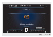
When on-board computer detects that the system is malfunctioning or its information is abnormal, the alarm information will be immediately displayed in information display area one by one and recorded in fault information screen after switching vehicle power to ON mode.
