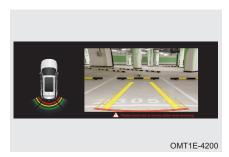
Move shift lever to R to enter parking view monitor screen, and the screen will display the parking view monitor and land guideline. Land guideline varies depending on steering wheel rotation and it is used for prejudging the reversing traveling trace.
