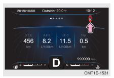
It is used to indicate opening/closing condition of door in any side.
