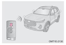
When the vehicle is in fortifying state and invalid entry is detected (such as any door or back door is opened invalidly, alarm will be activated), the vehicle will enter cyclic alarm mode, anti-theft horn sounds and turn signal lights flash. Press unlock button on smart key or switch vehicle power to ON mode to deactivate alarm.
