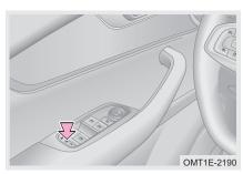
Press passenger side window OFF switch, passenger side window OFF switch indicator comes on, passenger side window switch will be disabled and the power child lock (if equipped) is locked. After disabling, only window switches on driver side can be used to operate passenger side windows (this function is recommended when there is a child in vehicle). Press the switch again to cancel this function and the indicator goes off.
