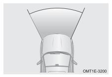
Operating conditions: In general, in a event of frontal collision, the driver airbag and front passenger airbag will deploy if the deceleration of vehicle exceeds the designed threshold level.
