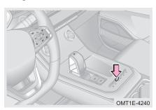
■ Entering panoramic view monitor When vehicle power is turned to ON mode and speed is < 15 km/h (D position): If parking radar obstacle distance signal is received, it enters panoramic view monitor system (if it is equipped with auto parking assist system (APA)).
