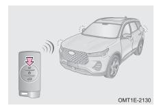
Press unlock button on smart key or touch the unlock sensing area with four fingers or approach vehicle when carrying smart key on your person, the system automatically recognizes validity of smart key and doors automatically unlock, the vehicle will exit fortifying mode.
