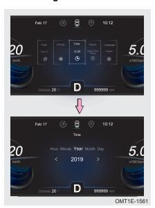
Time can be set by operating steering wheel combination buttons:
