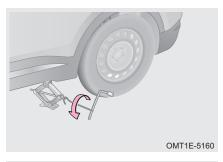
Step 3: Make sure all persons around the vehicle stay in the safe area, fit jack rocker into jack, and wheel bolt wrench into jack rocker, and turn wheel bolt wrench counterclockwise to lower the vehicle;
