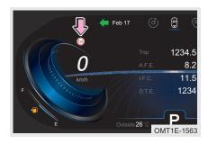
When speed reaches the set value, alarm icon "22" will be displayed on driving information display screen (specific set speed value will be displayed in the icon) and alarm buzzer sounds, the speed value turns red at the same time. Alarm icon and sounds will disappear only when speed is lower than setting value by 5 km/h. If speed reaches the set value again, it will alarm again.
