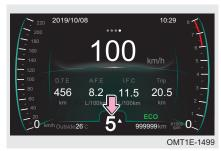
Display the currently selected gear position information (the current gear position in manual mode).
