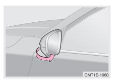
Hold the outside rear view mirror, and push it to the backward firmly and slowly (force increases gradually from small to large), until it folds to its position; Hold edge of the outside rear view mirror, and pull forward slightly, until it extends in place.
