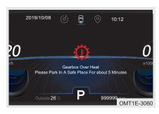
When the transmission temperature is high, the meter alarm text message is "High transmission temperature, stop at a safe place".
