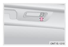
Press second row dome light switch, the second row dome light comes on, press again to turn it off.
