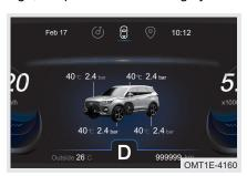
Steering wheel left combination button " ◀ "/right combination button " ▶ " can be used to switch to tire pressure display screen.
