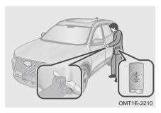
Method 1: Touch the lock sensing area with fingers when carrying smart key on your person, the system automatically recognizes validity of smart key and doors automatically lock.
