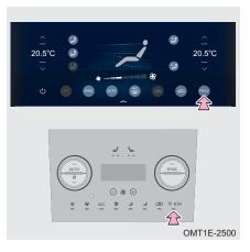
Operate the anion button on air conditioning control panel to enable the one-button purification function of air conditioning system to purify the air inside the vehicle.
