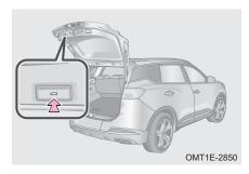
When the power back door opens, press the button  $\iff$  to close the power back door.
