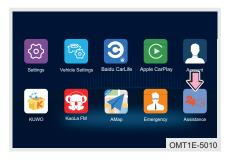
Manual vehicle emergency rescue: When an accident occurs, press soft button on the audio head unit, vehicle manually calls Chery customer service to ask for rescue, making travel more assured.
