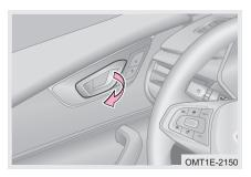
When doors are unlocked, pull door inside handle simply to open door.
