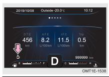
When driving time exceeds the set time, "Driving time exceeds--h, take a rest" will be displayed on information display area, at the same time, alarm sounds for 1 second and fatique driving icon displays "5" to inform the driver to take a rest.
