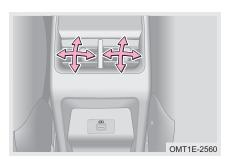
Move outlet adjustment lever up, down, left or right by hand to adjust direction of airflow.
