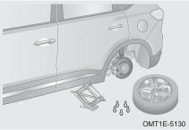
Step 5: Remove the wheel bolts of flat tire counterclockwise with the wheel bolt wrench, and remove the flat tire.
