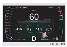
Driving mileage: The estimated maximum distance that can be driven with current remaining fuel (common unit: km).
