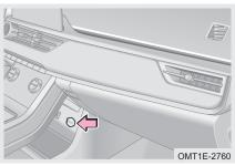
For some models, power outlet is located on the front end of auxiliary fascia console.
