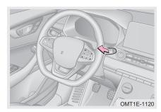
Turn vehicle power to ON mode, pull wiper combination switch towards the steering wheel and hold, the front washer sprays water, and front wiper operates simultaneously. Front washer will stop operating when the switch is released, the wiper will wipe 3 cycles at low speed, and operate one cycle then stop after a few seconds.
