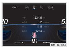
Display the currently selected gear position information (in manual mode or the current gear position).
