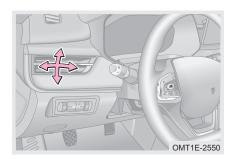
Move side outlet adjustment lever up, down, left or right by hand to adjust direction of airflow.
