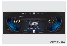
When tire temperature is > 85°C, and drives at a speed greater than 30 km/h for period of time, system will warn for high temperature. During high temperature warning, corresponding wheel icon will blink, current temperature value will be displayed and "!" yellow indicator in instrument cluster comes on.
