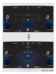
ESP function can be set by operating steering wheel combination buttons:
