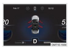
It is used to indicate opening/closing condition of door in any side or hood.
