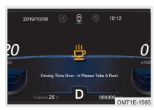
When driving time exceeds the set time, "Driving time exceeds X, take a rest" will be displayed on information display area, at the same time, alarm sounds for 1 second and fatigue driving icon displays "5" to inform the driver to take a rest.
