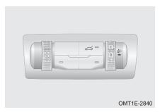
While vehicle power is switched to OFF/ACC/ON mode, shift the lever P position and the vehicle is in deactivation mode, long press the power back door switch, turn signal lights will come on and power back door will be opened/closed.
