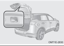
Pull the back door assist handle down and release it before the back door is fully closed. Make sure the back door is fully closed before leaving the vehicle.
