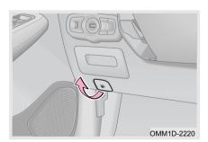
Step 1: The fuel tank cap will spring out by pulling fuel tank cap release lever:
