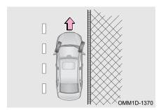
If there is curb on roadside, turn steering wheel to right by a certain angle to make front part of front right wheel close to or against the curb, to prevent vehicle from sliding forward along the slope, then apply the park brake.
