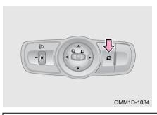
Operate using switch: When vehicle power is turned to ON mode, press outside rear view mirror folding switch to fold mirrors automatically, press the switch again to extend mirrors automatically.
