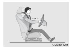
The shoulder belt should be over the shoulder center and close to the chest, kept away from the neck, the lap belt should be closed to the hips but not stomach.
