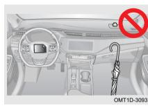
Do not attach anything to or lean anything against the areas such as the instrument panel, steering wheel and lower portion of the instrument panel. These items can become projectiles when driver frontal airbag or front passenger frontal airbag deploys.
