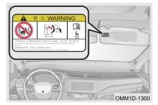
This sticker is attached to front passenger sun visor and used to remind you that the vehicle is equipped with front airbags. Observe the following precautions:
