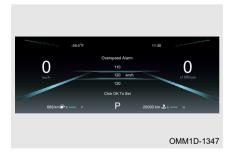
On overspeed alarm setting screen, press steering wheel combination button " ok " upward and downward to adjust the speed limit. Press " ok " briefly to set. Press steering wheel combination button " • " briefly to exit overspeed alarm setting.
