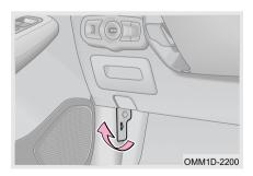
Step 1: The hood will spring up slightly by pulling hood release lever;
