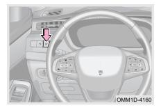
Click " " switch, idling stop-start system is disabled; Click " " switch again to enable stop-start system.
