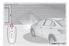
Turn vehicle power to OFF mode, press unlock button on smart key to activate the smart vehicle locating function. The low beam lights and position lights will come on for 60 seconds. Press unlock button on smart key again for a delay of 60 seconds.
