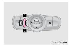
Headlight leveling adjusting switch includes 4 positions (0, 1, 2, 3), and it can be adjusted according to occupant quantity and vehicle load.
