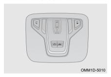
Manual rescue: When an accident occurs, manually press SOS button on the right (the left side is indicator display) to make an emergency call and start emergency rescue assist function.
