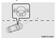
When speed increases to ≥ 65 km/h, LDW enters activating; When speed decreases from more than 65 km/h to 60 km/h, LDW enters preactivating; When speed is < 60 km/h, LDW exits after 3 seconds.
