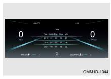
On time setting screen. press steering wheel combination button " ok "upward and downward to adjust time. Press " ok " briefly to set (in year/month/date/hour/ order Press steering minute). wheel combination button " ◀ " briefly to exit time setting.
