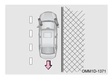
If there is curb on roadside, turn steering wheel to left by a certain angle to make rear part of front right wheel close to or against the curb, to prevent vehicle from sliding backward along the slope, then apply the park brake.
