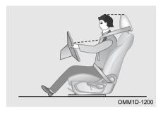
When sitting, slightly incline rearward (25° backward from vertical position is proper) and well back on seatback.
