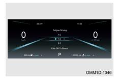
On fatigue driving setting screen, press steering wheel combination button " ok " upward and downward to adjust reminding time. Press " ok " briefly to set. Press steering wheel combination button " ◀ " briefly to exit fatigue driving setting.
