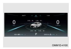
On driving information screen, move steering wheel combination button " ok " upward and downward to tire pressure display screen, then tire pressure and temperature values can be checked.
