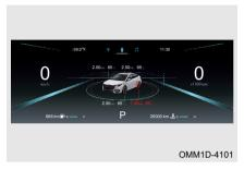
When tire pressure is < 1.92 bar, and drives at a speed greater than 30 km/h for period of time, system will warn for low pressure. During low pressure warning, corresponding wheel icon will blink, current tire pressure value will be displayed and "(!)" yellow indicator in instrument cluster remains on.
