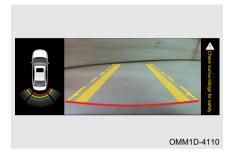
Move shift lever to R to enter RVC screen, and the screen will display the parking view monitor and lane guideline. Lane guideline varies depending on steering wheel rotation and it is used for prejudging the reversing traveling trace.
