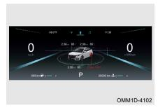
When tire temperature is > 85° C, and drives at a speed greater than 30 km/h for period of time, system will warn for high temperature. During high temperature warning, corresponding wheel icon will blink, current tire temperature value will be displayed and "!" yellow indicator in instrument cluster remains on.
