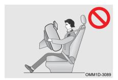
Always keep airbag (SRS) inflation path clear. It is forbidden to place anything (such as mobile phone, etc.) between the occupant and the airbag (SRS). It is forbidden to fix or place any object on or near the airbag cover. If there is an object between occupant and airbag (SRS), the airbag (SRS) may not deploy according to design path, or the airbag (SRS) may push object to occupant's body, causing serious injury or even death.
