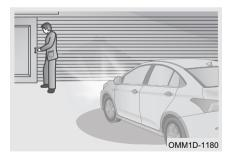
ON: Turn vehicle power to OFF mode, pull the headlight combination switch towards steering wheel side and release within 2 minutes, the follow me home function is activated. The low beam lights and position lights will come on. Each time the headlight combination switch is operated, the low beam lights and position lights will turn on for 30 seconds, which can be activated up to 8 times continuously.
