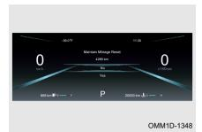
screen, press steering wheel combination button " ok " upward and downward to YES/NO. Press " ok " briefly to set. Press steering wheel combination button " \( \blacktriangle \) " briefly to exit maintenance mileage reset.
