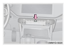
In case of vehicle failure or traffic accident etc., please turn on the hazard lights to warn other vehicles to avoid the secondary accident.
