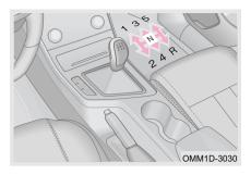
Step 1: Depress the clutch pedal and brake pedal completely, then shift the shift lever into proper gear;
