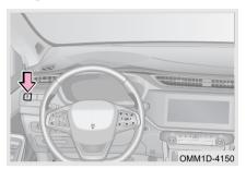
Press " witch (if equipped) to turn off ESP; Press the " witch (if equipped) again to turn on ESP.
