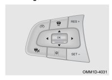
When " utton is pressed. TJA/ ICA is turned on and ACC is turned on automatically at the same time, " gray indicator in instrument cluster remains on. When all ACC activation conditions are met, press "SET-" button. ACC is activated firstlv. meanwhile. front detect if there are lane lines or vehicle targets, when activation conditions are met, green indicator in instrument cluster remains on.
