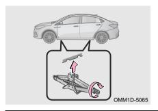
Step 3: Place jack on firm and level ground, turn jack handle clockwise by hand, making the notch of jack contact with the correct jacking-up point;
