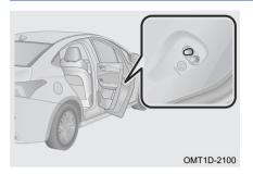
The child-protection lock is located at inner side of rear doors.
