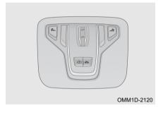
Press "&\$" switch when moon roof is closed, the moon roof will tilt up.
