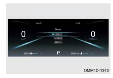
On theme setting screen, press steering wheel combination button " ok " upward and downward to adjust theme. Press " ok " briefly to set. Press steering wheel combination button " ◀ " briefly to exit theme setting.
