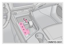
Step 1: Depress the brake pedal completely and press button on shift lever, then shift the shift lever from P to D:
