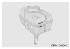
When engine is cold, the coolant level should necessary to between the "MIN" and "MAX" marks. If the level is in the "MIN" mark or below, add coolant.
