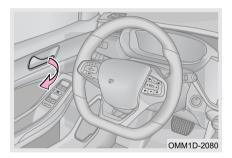
When doors are unlocked, pull door inside handle simply to open door.
