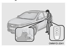
Method 1 (if equipped): Press microswitch on door handle when carrying smart key, the system automatically recognizes validity of smart key and doors automatically lock.
