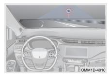
After SLA detects speed limit sign information on road in front and combines the information with speed limit information of navigation system, " (20)" indicator in instrument cluster remains on, if the speed exceeds current speed limit for 5 km/h, prompt sound will sound 1 time.
