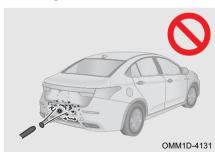
When washing vehicle, use a soft cloth or water (low water pressure) to wash off foreign matter such as snow, mud, and dust on the surface of the radar sensor.
