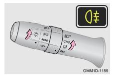
Turn vehicle power to ON mode, when low beam lights turn on, turn fog light knob to " 0‡ " position to turn on rear fog lights; After turning vehicle power to OFF mode or turning fog light knob to " 0‡ " position again, rear fog lights turn off.
