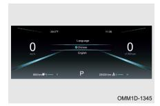
On language setting screen, press steering wheel combination button " ok " upward and downward to adjust language. Press " ok " briefly to set. Press steering wheel combination button " ◀ " briefly to exit language setting.
