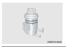
Brake fluid level should be between the "MIN" and "MAX" marks. If the level reaches the "MIN" mark or below, add brake fluid.
