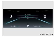
On ESP function setting screen, press steering wheel combination button " ok " upward and downward to ON/OFF. Press " ok " briefly to set. Press steering wheel combination button "
